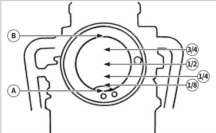
**Effect of setting parts in relation to throttle valve opening (XX 125 / XX 250 versions)**
