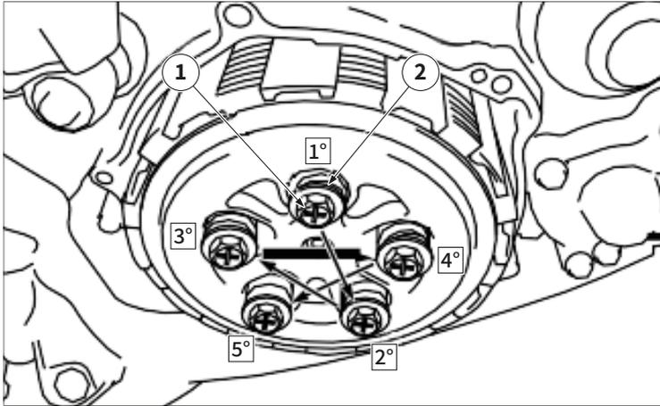
Remove bolts “1” and springs “2” of the clutch following a cross pattern;
