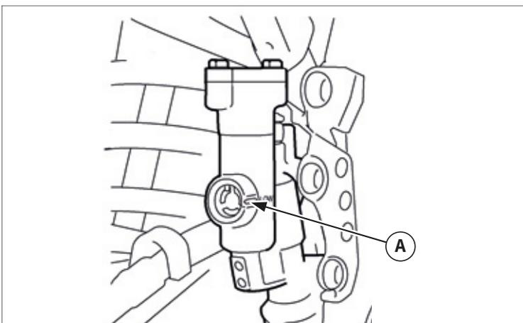
**Check the rear brake fluid level**
