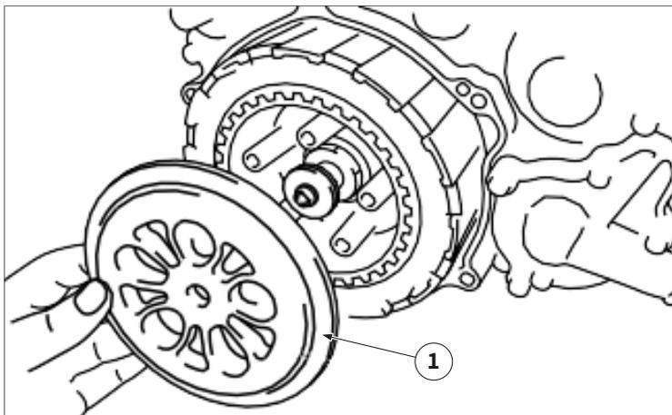
– Remove the pressure plate “1”;
