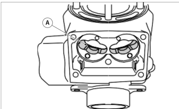
Remove carbon deposits from power valve hole surface "A".
