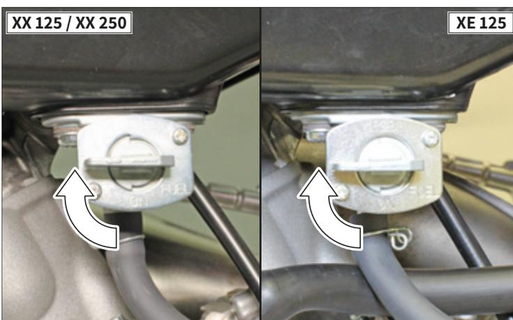
**⚠ Always set the fuel cock to OFF when the engine is switched off.**
