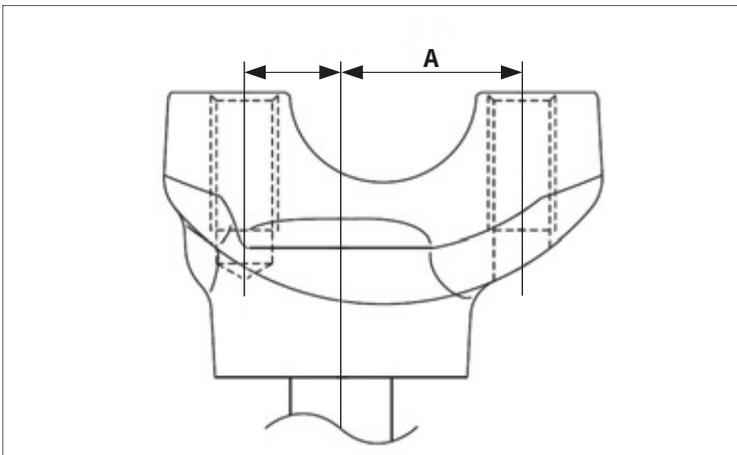
**!** Install the lower handlebar mounts so that the side with the longest distance "A" faces forward. By installing them in the opposite direction, it is possible to change the front/rear off-set of the handlebar position.
