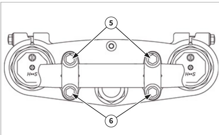
First tighten the bolts on the front side "5" of the upper handlebar holder, and then tighten the bolts "6" on the rear side.
