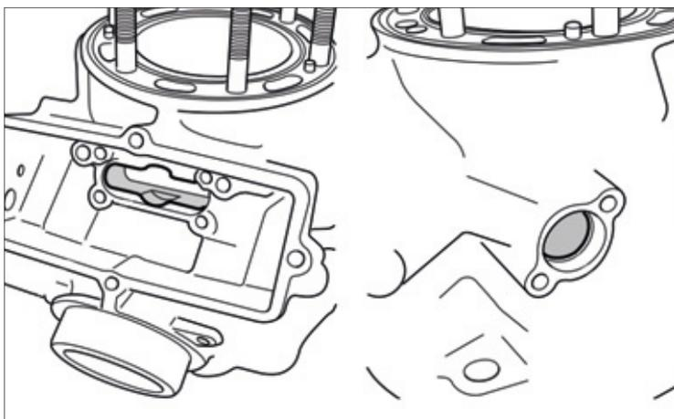
Remove carbon deposits from the surfaces of the exhaust valve seats.
