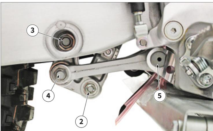
– Regularly check the shock absorber lower fastening screw “2” and linkage fastening screws “3”, “4” and “5”. If they are loose, tighten them to the specified torque.
